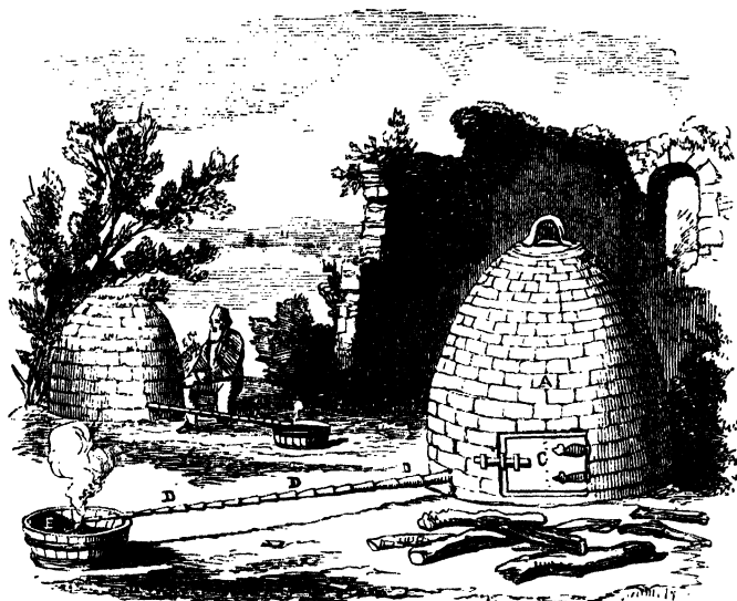
Fig. 91. Glauber's Method of procuring Acetic Acid by the destructive Distillation of Wood, copied from his "Miraculum Mundi." "A is the Furnace or oven, wherein the wood is char'd. B. The Cover of the Furnace. c. The door at which the coals are taken out. D. The Canes or Pipes wherein the sap or juice of the wood is condensed, and from thence runs into the receiver. E is the vessel or receiver into which the vinegar of wood runs."
